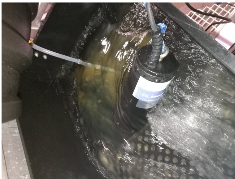
Figure 3.9: The Franatech handheld sensor measuring in the side wall drain of tank 1 in Veksthall 1 at Nofima.
