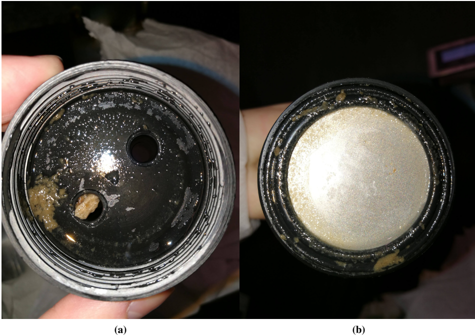
Figure 4.12: The Water-pumped flow-through head (a) and Teflon membrane (b) after part 2 of the experiment. The head was washed with tap water for 30 minutes before detaching the pumped head.
