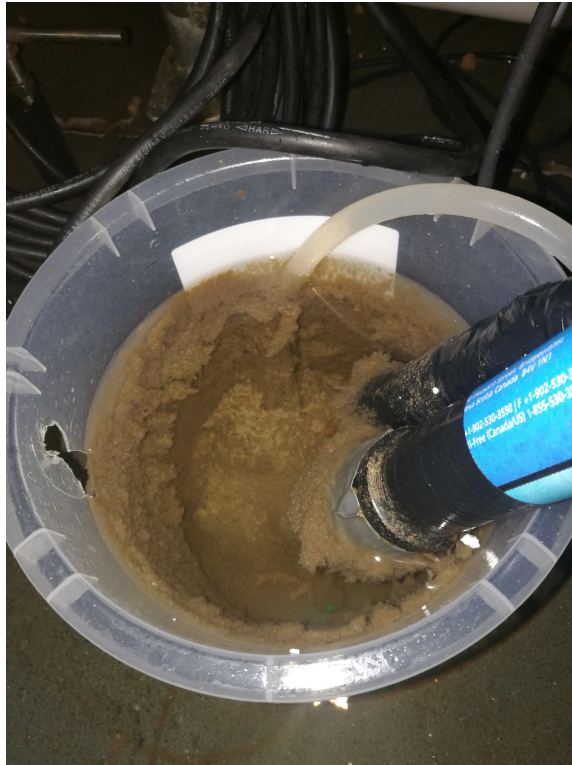
Figure 4.18: Sedimentation in the by-pass after two weeks of the experiment.
