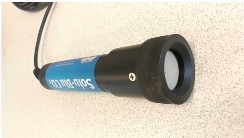
Figure 3.1: Pro-Oceanus Solu-Blu dissolved carbon dioxide ( \text{CO}_2 ) sensor with the open faced head and Teflon membrane.
