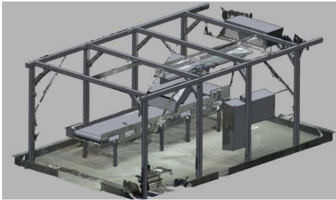
Fig. 7 Hybrid model of point cloud, mesh, and solid models in Design X
