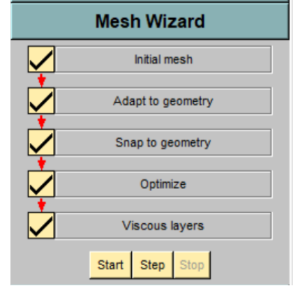
Figure 15: 5 steps of meshing process in FINE/Marine
