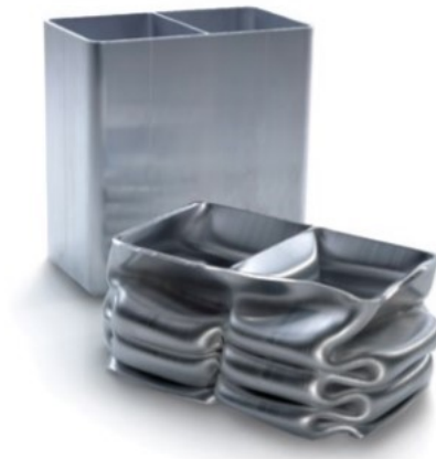
Figure 1.1: Crash component before and after deformation. Image from [2]
