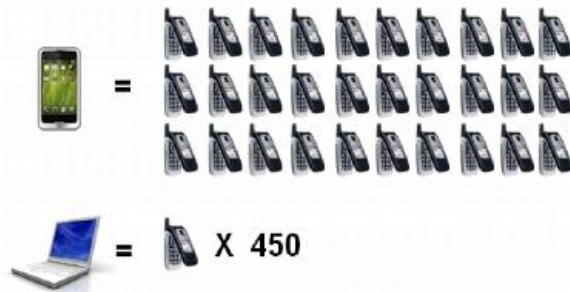
Figure 2-3. Full-successful smartphones (i.e. Iphone and similar) can generate as much traffic as 30 basic-feature voice-based phones, new high-end handsets and laptop cards as much as 450 basic-feature phones
