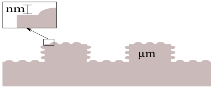
Figure 2.5: Illustration of a hierarchical structure containing nanosized asperities on top of microsized asperities, providing a nanoroughness and microroughness respectively.
