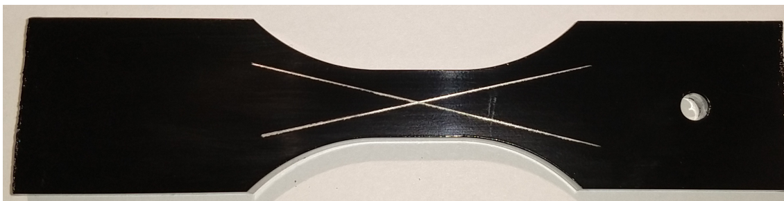
Figure 3.8: A scratched KTL sample ready for corrosion fatigue testing.
