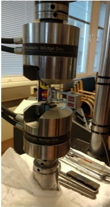
Figure 19 - Tensile test setup for MTS 810 Hydraulic Tensile testing machine.
