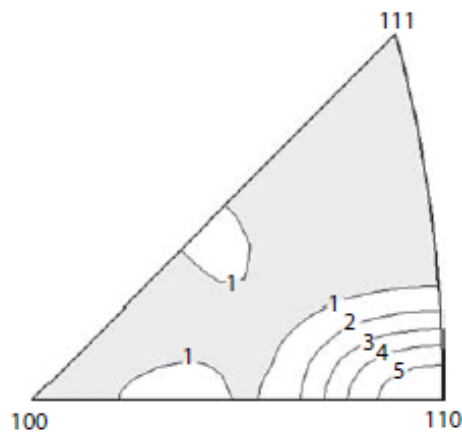
Figure 11 - Inverse pole figure of pure uniaxially compressed copper. There is a significant amount of \langle 110 \rangle fiber, with some \langle 210 \rangle fibers as well. (Engler & Randle, 2010)
