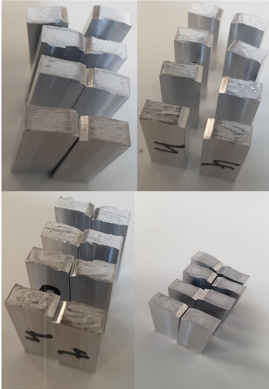
Figure 96 - Pictures showing the Charpy samples for 0-39.1%CW of AA7090. Cold work increases from left to right and from top to bottom.
