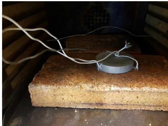
Figure 26 - Setup with a thermocouple inside the sample and a thermocouple in the air just above the sample.
