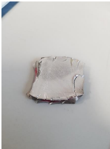
Figure 28 - Image showing cracks in a cubic sample cold pressed more than 70%.
