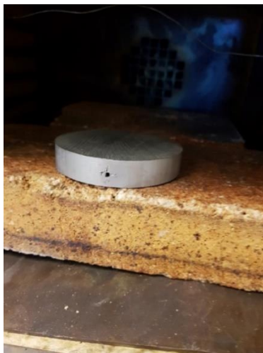
Figure 25 - The AA2196 sample piece used when measuring the temperature inside the alloy with respect to that of the furnace.
