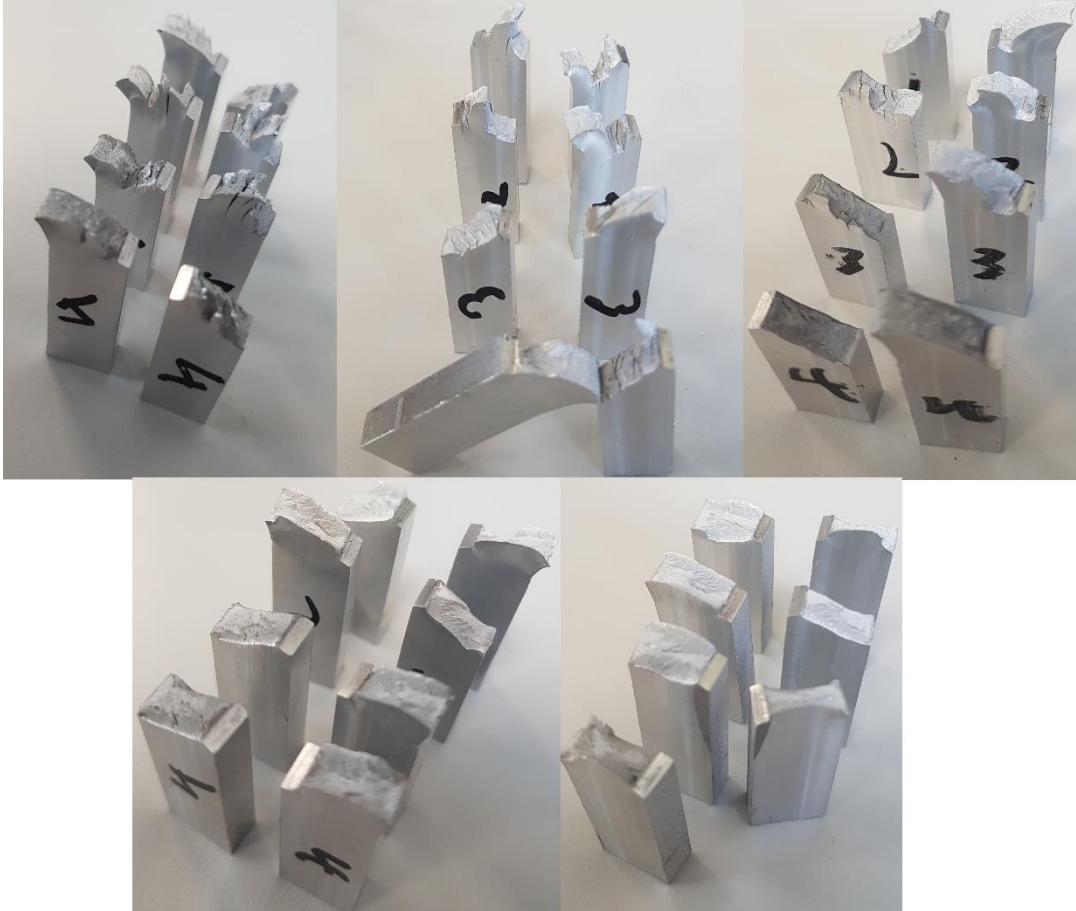
Figure 50 – The fracture surfaces of Charpy samples for 0-56.3%CW AA2196. Cold work is increasing from left to right and top to bottom.
