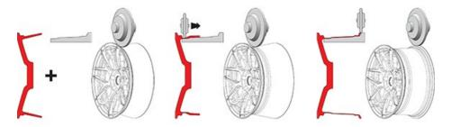
Figure 2.1: Flow Forming Schematic of Rim [11].
