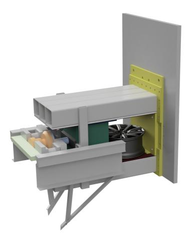
Figure 5.2: CAD model of the assembly with part of trolley and kicking machine rails.
