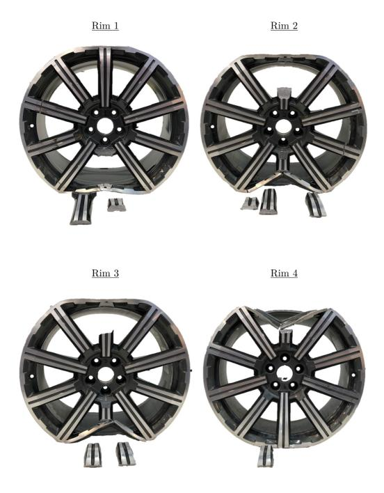
Figure 6.45: Images of all rims after testing. Impact from the bottom side of the images.
