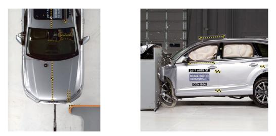
Figure 1.1: Small overlap crash test of the 2017 Audi Q7 [3].
