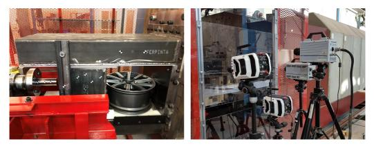
Figure 6.13: DIC overview and camera setup.
