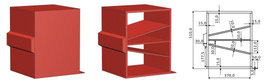
Figure 6.5: View and dimension of impact box with inner plates and impact plate.
