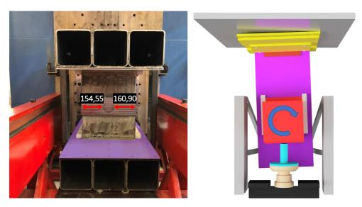
Figure 6.21: Off-centered impact. Figure 6.22: Exaggerated rotated test rig.
