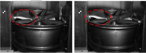
Figure 6.44: Rim 4. Visual deformation at given displacement.
