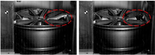
Figure 6.43: Rim 3. Visual deformation at given displacement.
