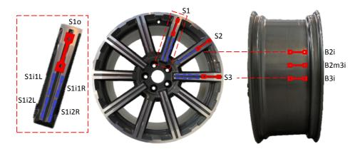
Figure 3.5: Where specimens are taken from. Red = Tensile specimens.Blue = SHTB specimens.
