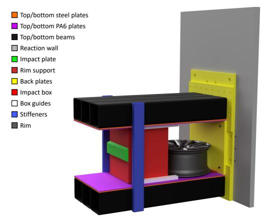
Figure 6.3: Crash rig assembly.
