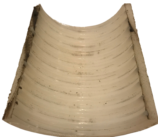
Figure 3.1: Part of a virgin PA11 liner used for the experimental work conducted in this thesis.
