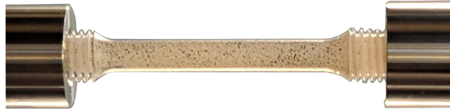
Figure 4.2: Illustration of how the specimens are fastened with threads (the picture is rotated 90 degrees).
