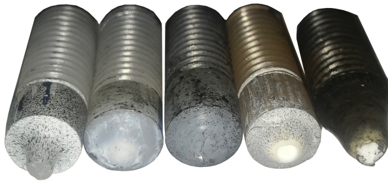
Figure 4.19: Fracture surfaces of a selection of test specimens. From left to right: V-R2-H, V-R2-C, P-R2-C, PW-R2-H, PW-R2-C.
