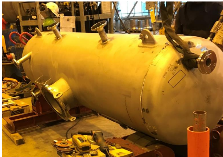
Figure 17: Pressure vessel with nozzles and brackets (With permission from case company)
