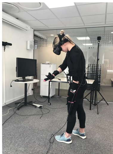
Figure 3.9: Operator wearing an IMU-MoCap suit while connected to HTC Vive.
