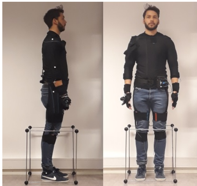
Figure 4.4: Male 3 standing inside the JIG used for skeleton calibration
