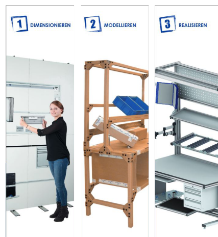
Figure 3.1: Three stages of a workstation design process. Visualisation, physical mock-up, CAD prototype and finished product. (Photo: https://www.cardboardengineering.de/ , access date: 06 june 2019)
