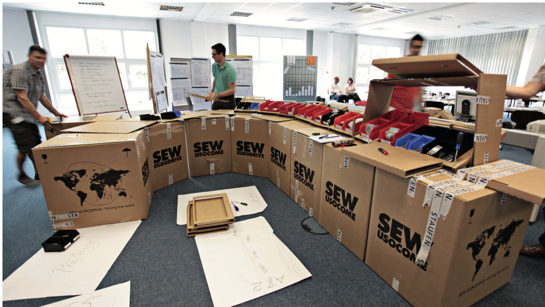
Figure 3.3: Engineers are creating a cellular workstation mock-up out of cardboard. (Photo: Staufen AG, URL: https://www.heise.de/select/ct/2019/8/1555071151816291 , Access date: 06 June 2019)
