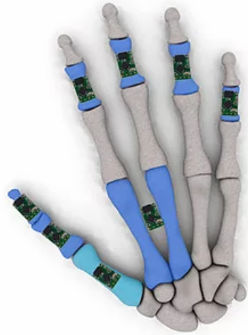
Figure 4.3: Sensor placing of the Cobra Glove ( www.synertial.com/gloves )
