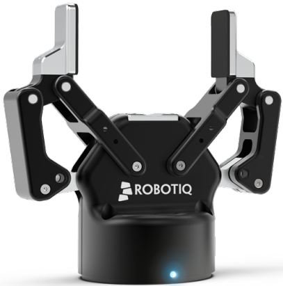
(c) Robotiq 2F-85 gripper [16]
