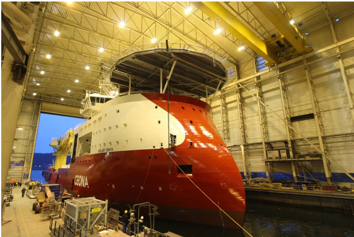
Figure 4: Launching of Polar Onyx from the dry-dock at UVE. An offshore construction vessel built with Ulstein X-BOW®. (Photo by: Tonje Øyehaug Ruud)
