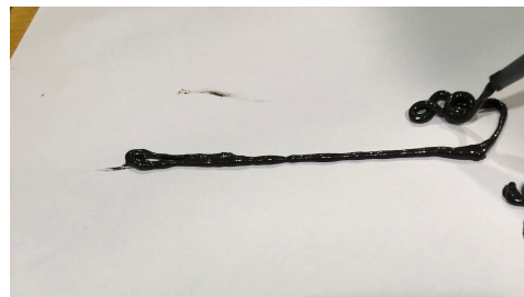
Figure 7.3: Sealant application errors.
