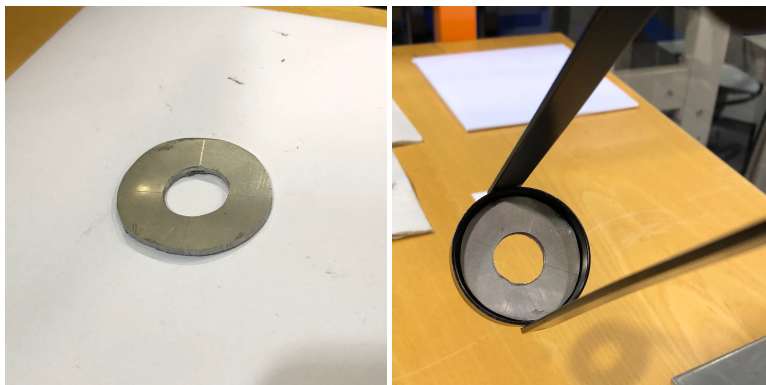
Figure 6.4: Flat metal ring solution to the caulking gun design flaw.
