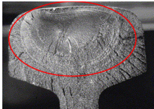
Figure 2.10: Kidney crack in traverse section (Steenbergen, 2016)
