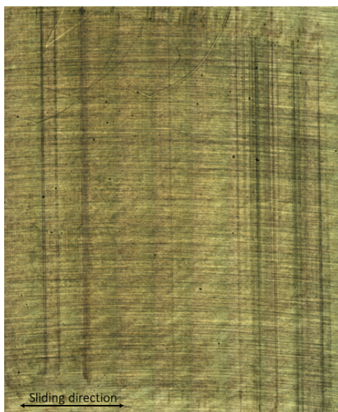
Figure 4.3: Wear track obtained on SDSS surface when cathodically protected after reciprocal sliding of a NAB cylinder for 1800 s at 0.01 m/s.
