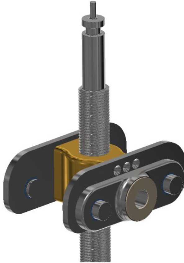
Figure 1.2: Illustration of the SDSS power screw with connected NAB nut. The power screw is coated with xylan 1052 coating.
