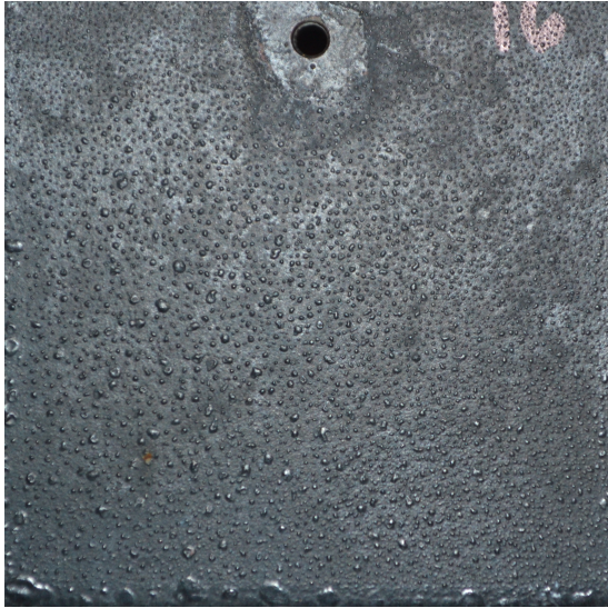
(a) Xylan surface after cathodic polarized by being coupled to a Zn-anode for 110 days.
