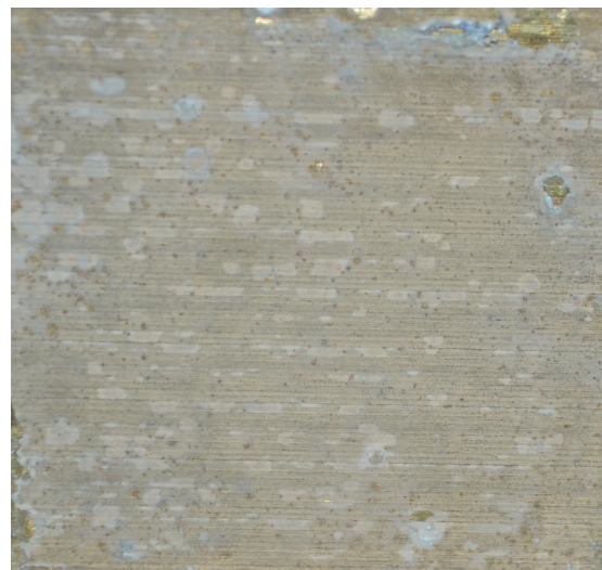
(b) NAB surface after cathodic polarized to -1050 \text{ mV}_{\text{Ag}/\text{AgCl}} for 157 days.
