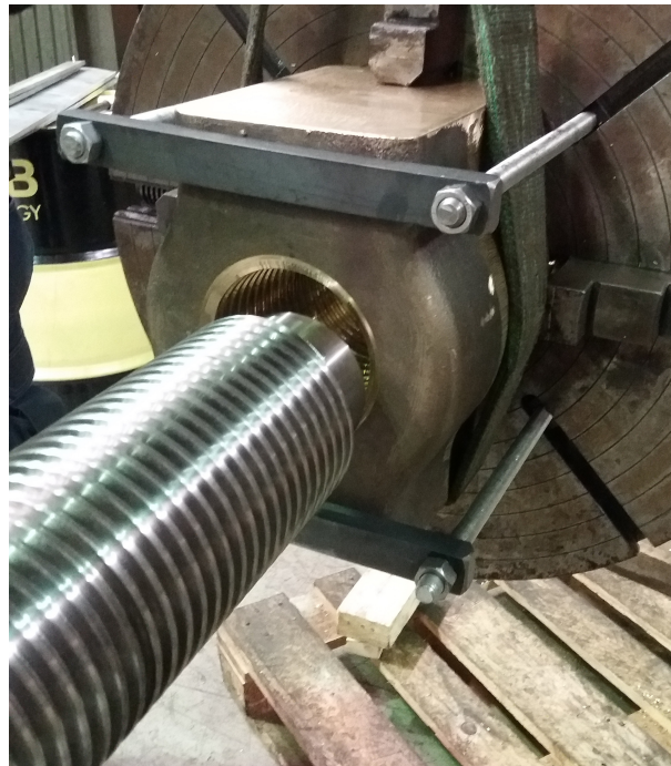
Figure 1.12: Photograph showing the uncoated SDSS power screw and the NAB nut.
