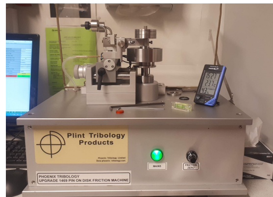
(b) Pin-on-disk tribometer used for dry continuous tribotests at different loads and speed.
