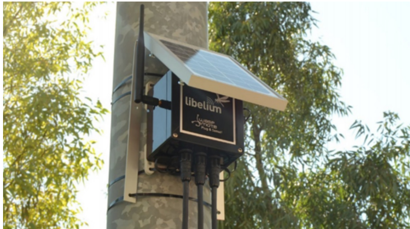
Figure 5: The Libelium Smart Water node together with the standard solar panel. Photo: Libelium (2019).
