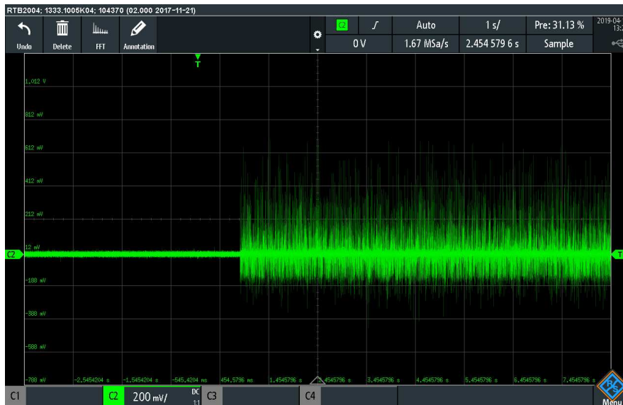
Figure 14: A constant low signal being distorted by the step-up converter. The oscilloscope used here is the Rohde & Schwarz RTB2004.
