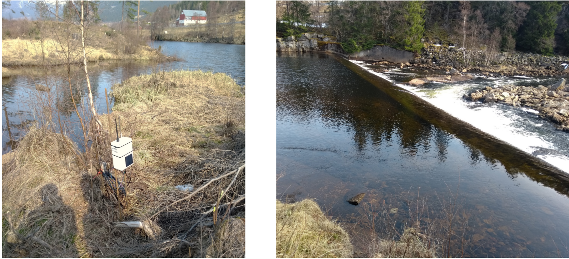
Figure 23: First field test. The picture to the right shows the node mounted to a thin steel rod. The picture to the right shows the threshold that depth measurements are calibrated to.
