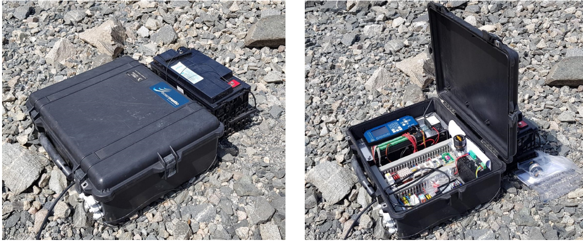
Figure 4: One of the Scanmatic depth measuring stations.
