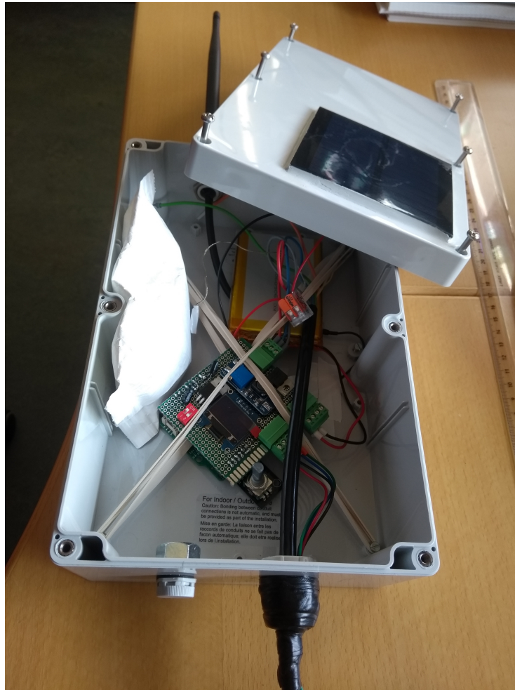
Figure 22: The prototype inside the temporary enclosure.
