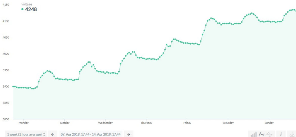
Figure 24: Battery voltage the first week of the test. AllThingsTalk Maker is used to display the data.
