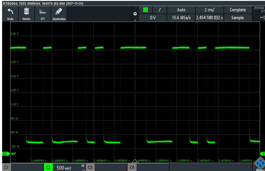
Figure 15: Communication between the microcontroller and the OTT PLS depth sensor. The wires have a distance of approximately 5 mm from coil of the step-up converter. No noise is detected.
