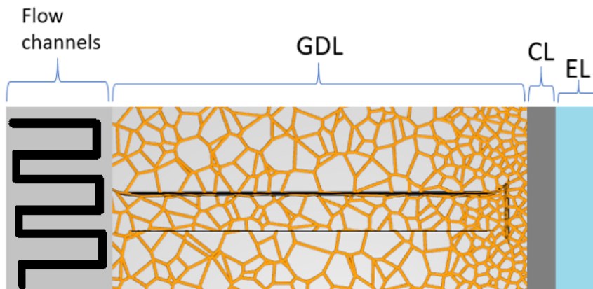
Figure 1.7: Interpretation of an "optimal" GDL (orange) featuring a porosity gradient and a large smooth channel for water transport (black)
