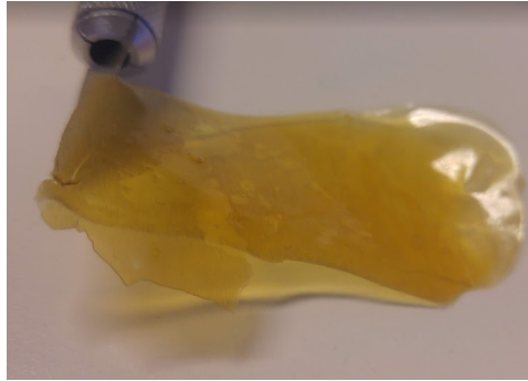
Figure E.7: PAA-resin after curing
