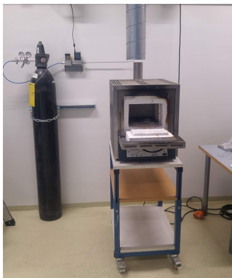
Figure E.9: The modified Lab Furnace used for imidization with attached Nitrogen and flow controller on the left.
