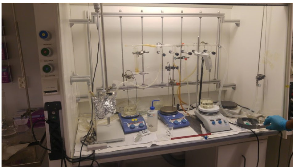
Figure E.4: Schlenk line setup used for synthesis
