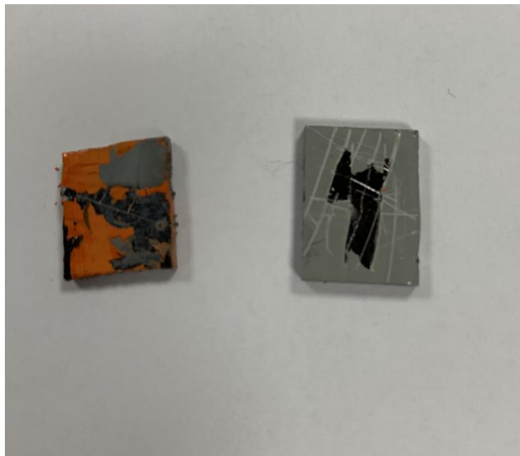
Figure 5.1: Removed paint with the use of liquid nitrogen. Test samples.
