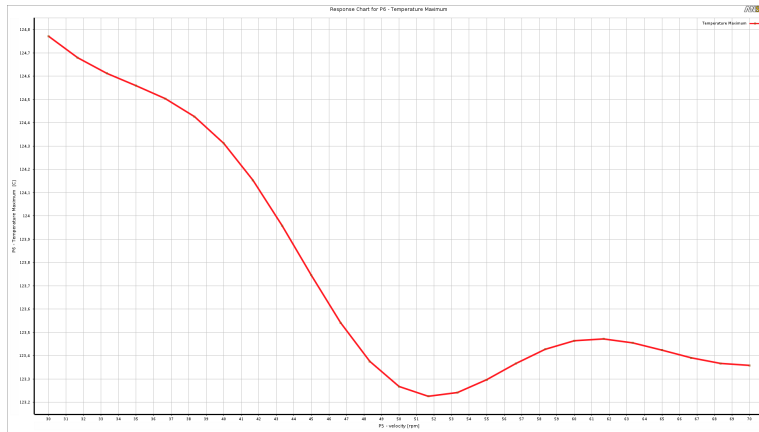
Figure 8.5: Generated response surface showing temperature over velocity.
