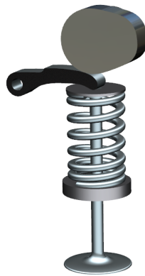
Figure 3.5: Simplified model of the relevant parts of the valve train.
