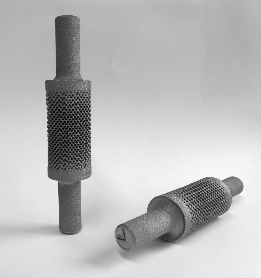
Figure 3.10: A batch of EBM manufactured Ti-6Al-4V fatigue specimen with TPMS D topology and variable volume fraction. The image show two specimen displayed from different angles.
