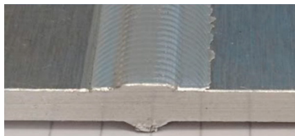
Figure 2.17: A dissimilar Al-Fe butt joint produced with the HYB process. The separate die on the housing makes it possible to control the shape of the weld face. Copied from [56].
