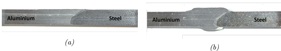
Figure 3.5: Photographs of selected tensile specimens prior to testing (a) flush-machined and (b) as-welded.
