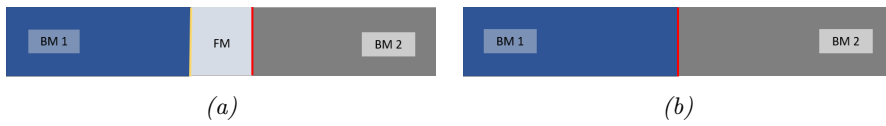
Figure 2.4: Depending on which joining technique that is used, different interfaces and bonding mechanisms can be observed. (a) illustrates the two interfaces that will form by the use of a filler material addition between BM1 and BM2, while (b) shows the one interface that appears by directly bonding the two metals.
