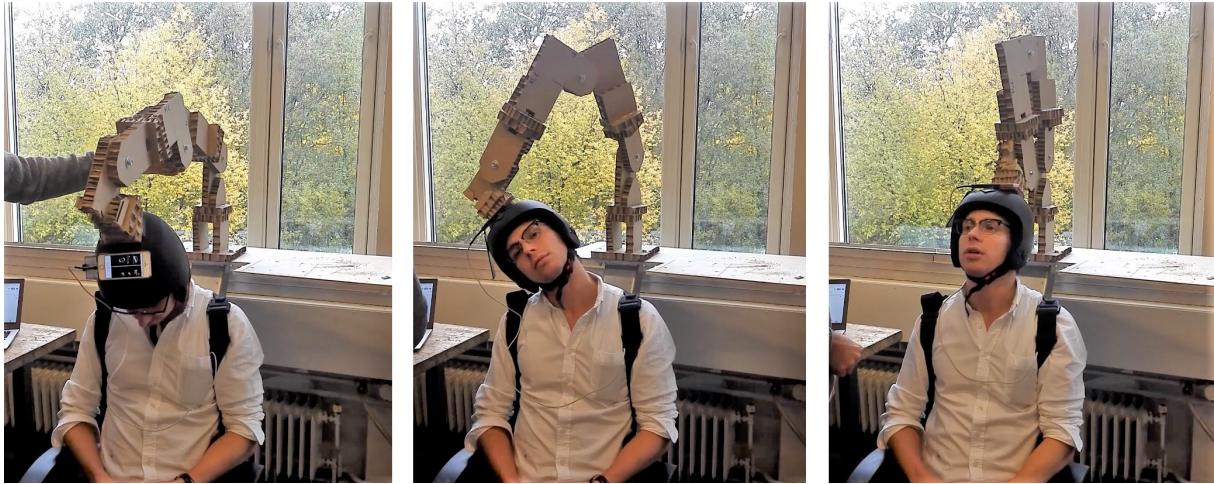
Figure 3.4: Three of the extreme positions of the head tested with the model attached in the original position
