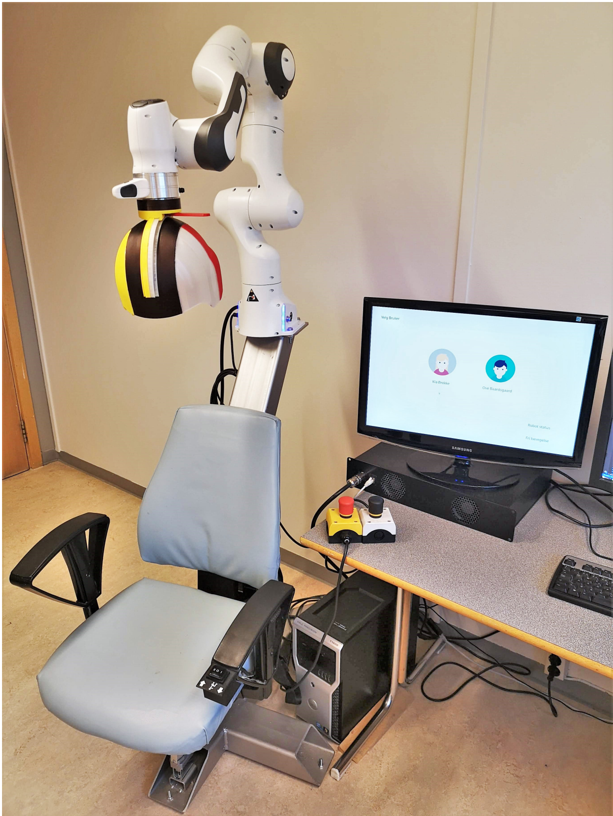
Figure 4.2: Current solution with the chair from the Brattgjerd and Festøy (2018) thesis, the Panda robot arm, helmet and magnetic connection, and the GUI start page.
