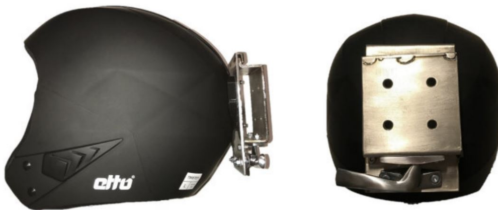
Figure 2.1: Mounting mechanism prototype(Brattgjerd, 2017)
