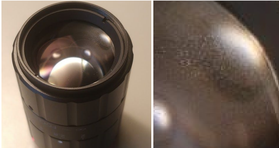
Figure 14: Unknown damage on 50 mm front lens
