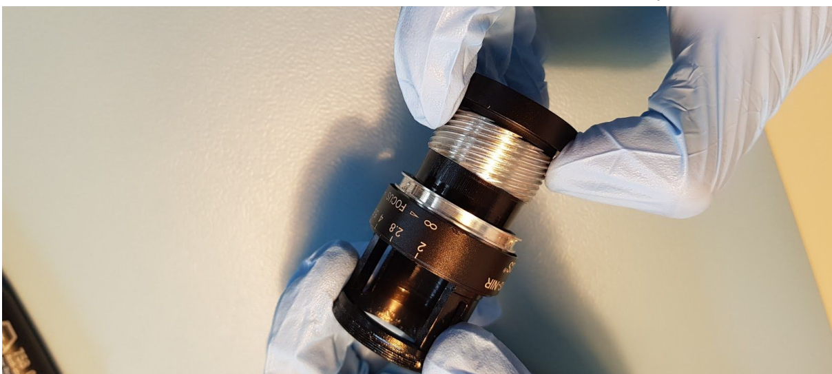
20. Separation of control unit from central lens assembly
