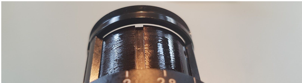
Figure 5: Grease inside the objective
