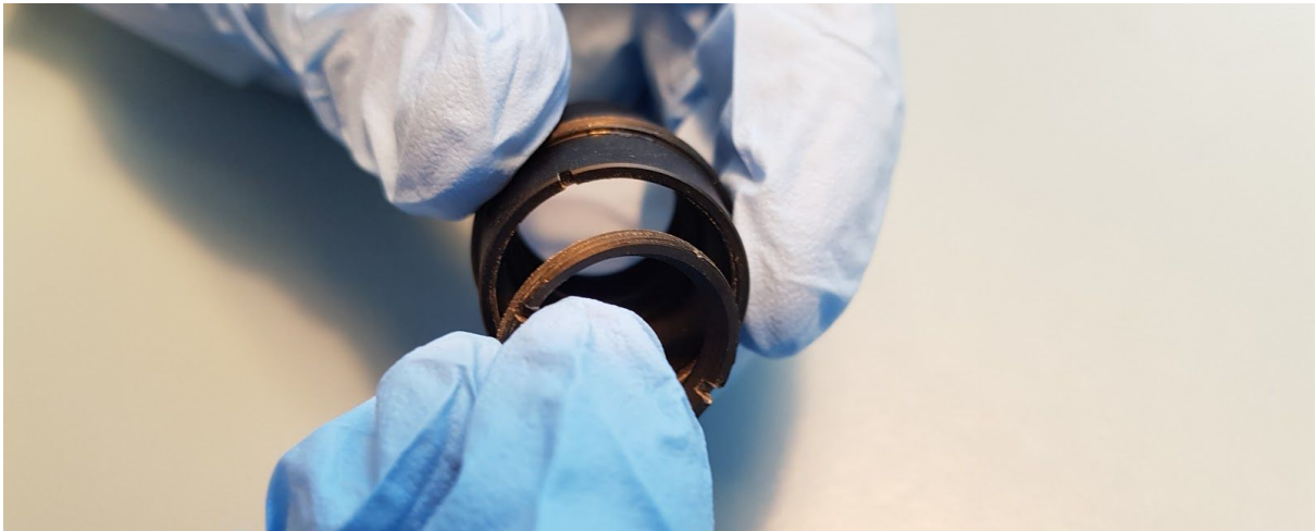
36. Removal of back end lens form the -Z lens tube
