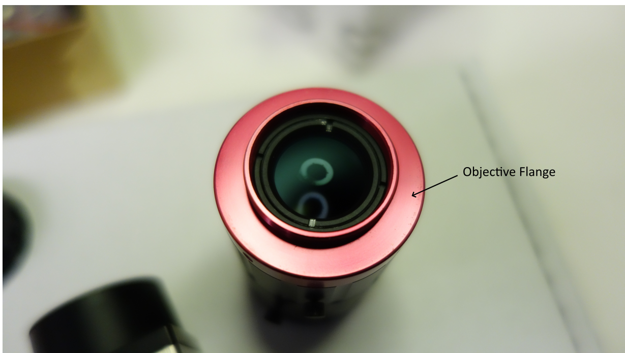
Figure 9: The flange surface on the Edmund Optics 50mm VIS-NIR objectives
