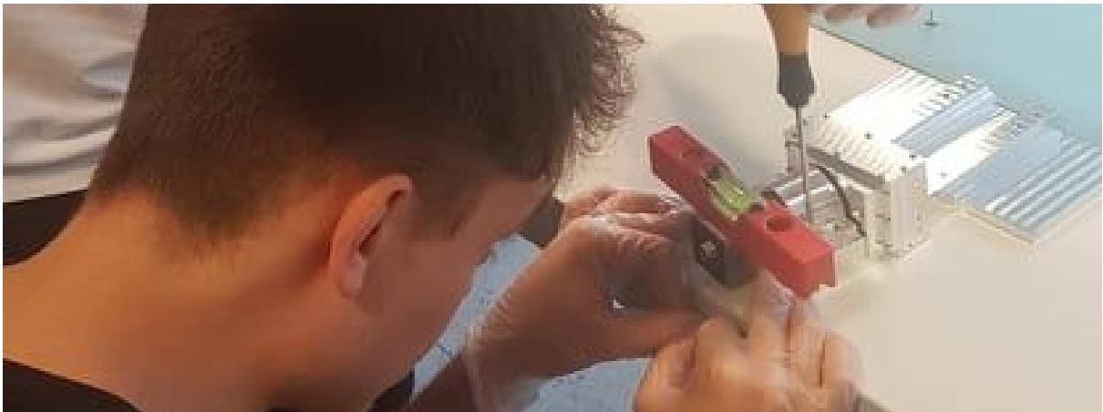
Use a level and fasten the bracket bolts incrementally on the back optics
