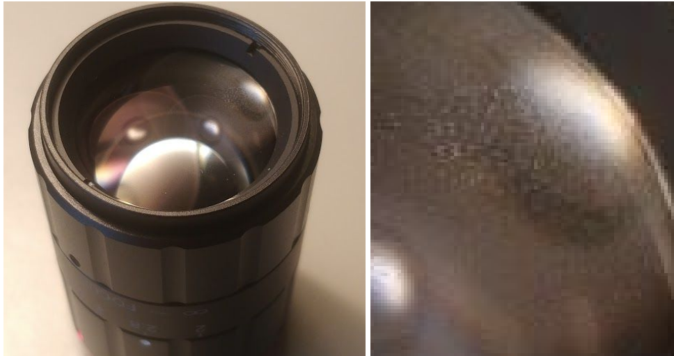
Figure 14: Unknown damage on 50 mm front lens
