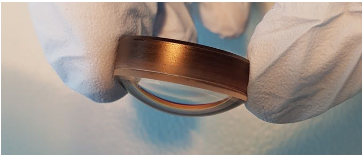
31. Middle lens with an apparent seam, appears to be glued
