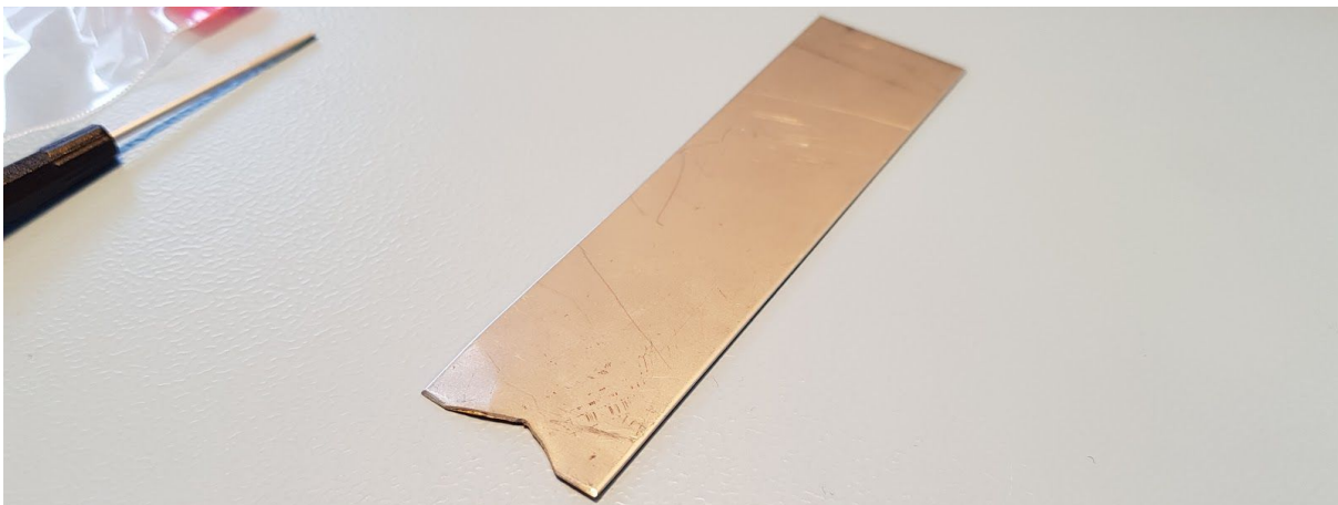
Figure 1: Custom 1 mm steel key plate
