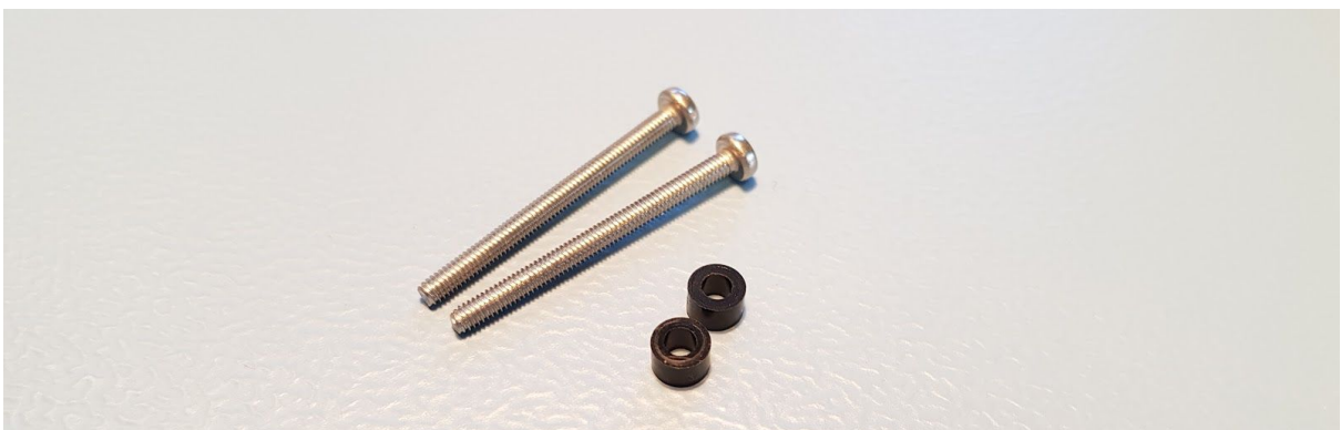
Figure 3: Ferromagnetic bolts and polymer washers
