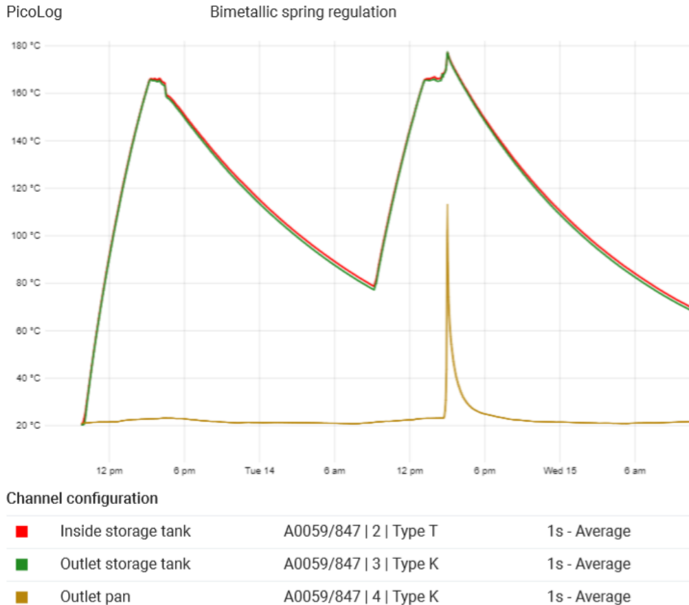
Figure 64: Test of bimetallic spring over 2 days
