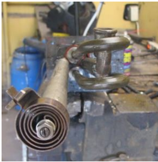
(a) The bimetalllic spring
