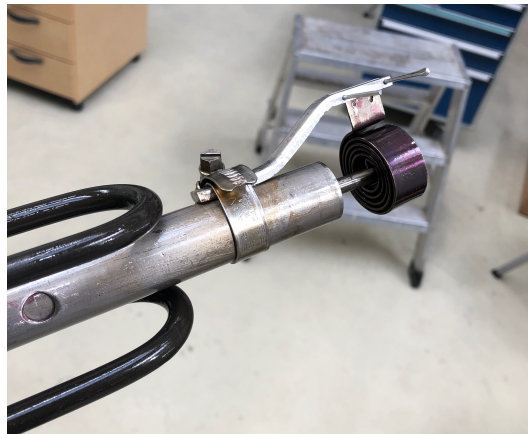
Figure 51: Bimetallic spring mounted on slider and pipe
