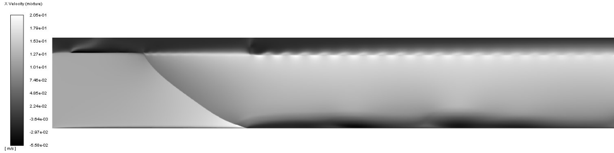
Figure 4.8: Velocity contour plot when a flow straightening porous region, modelling the effect of a honeycomb, is present downstream of the screen. Observe that the vortices present in figure 4.7 have almost disappeared. This contour plot is taken at the same time-instant as those in figure 4.7.
