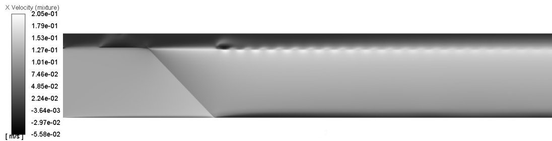
Figure B.14: Velocity contour plot resulting from the straight screen mounted such that the angle between the screen normal and the streamwise direction is \theta = 44^\circ at a flow time of 15s.
