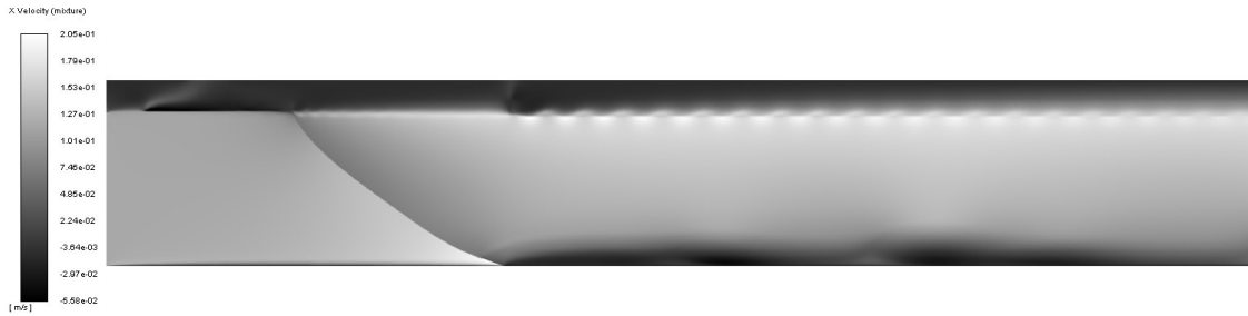
Figure B.16: Velocity contour plot resulting from the lab set-up using a water depth of 0.08m at a flow time of 15s.
