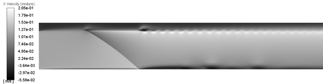
Figure B.7: Velocity contour plot resulting from the concave screen with a radius of curvature of 0.6m at a flow time of 15s.
