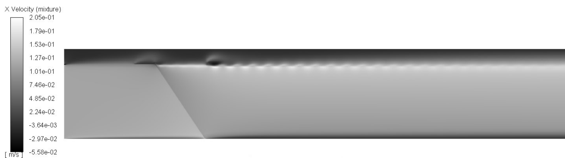
Figure B.15: Velocity contour plot resulting from the straight screen mounted such that the angle between the screen normal and the streamwise direction is \theta = 34^\circ at a flow time of 15s.
