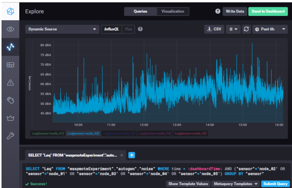
Figure 2.5: View of the Chronograf dashboard. A query is submitted to InfluxDB, and a graph is plotted from the results. The time interval can be adjusted in the top right corner.
