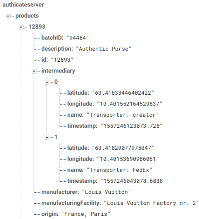
Figure 7.2: JSON-object structure stored on Firebase
