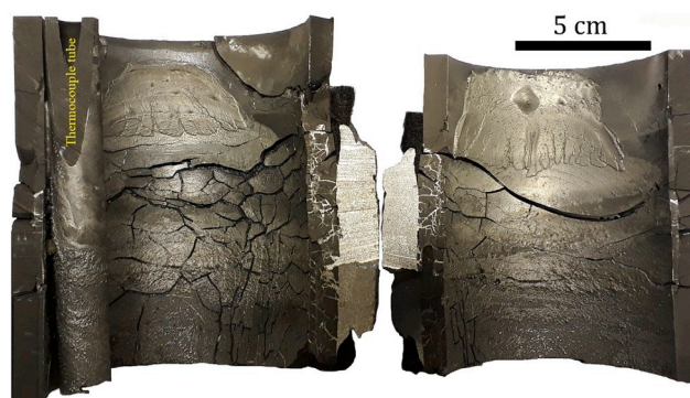
Fig. 6. The photograph of the graphite crucible after adding Al to Si at 1500 °C. The crucible burst immediately after the alloying process.
