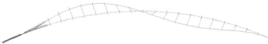
(a) First sway mode shape with eigen period of T_p = 56.72 s
