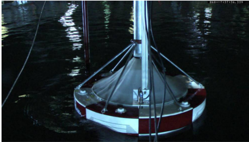
Figure 2: IEA OES Task 10.2 float geometry. The picture is retrieved from [10]
