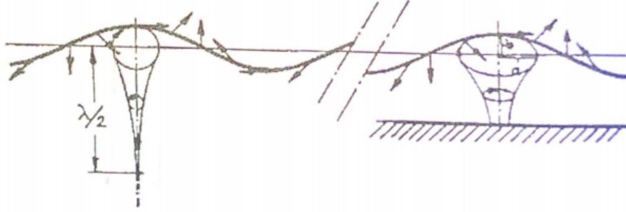
Figure 11: Movement of a water particle at the free surface in deep and finite water. Retrieved from [47]
