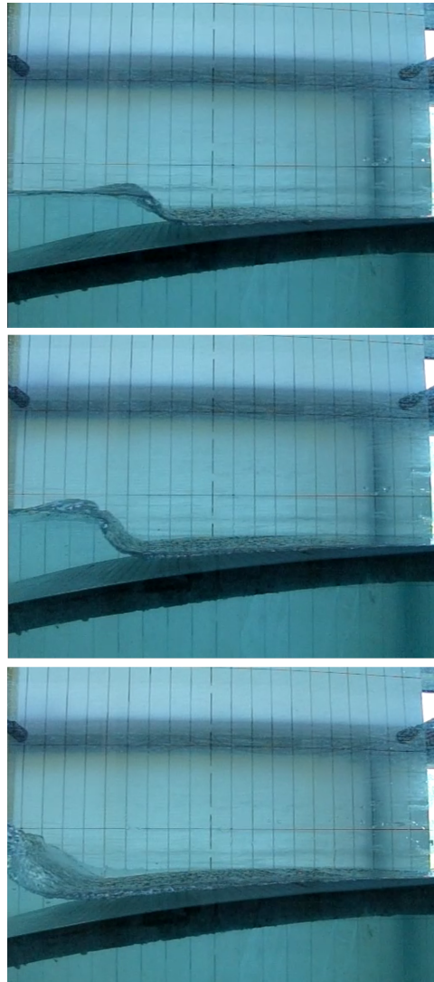
Figure 4.18: Comparison of observed point of breaking for waves with full scale wave period of 12 seconds and with top of beach at z = 0.00 for three different steepnesses. From the top and down: s = 1/60 , s = 1/45 and s = 1/30 .
