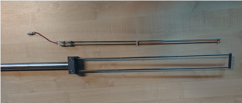
Figure 4.6: The two types of wave probes used. The upper wave probe type was used for the experiment in the Small Towing Tank and the lower wave probe type was used for the experiments in the Lader Wave Laboratory. The lower one was found to be the most accurate.
