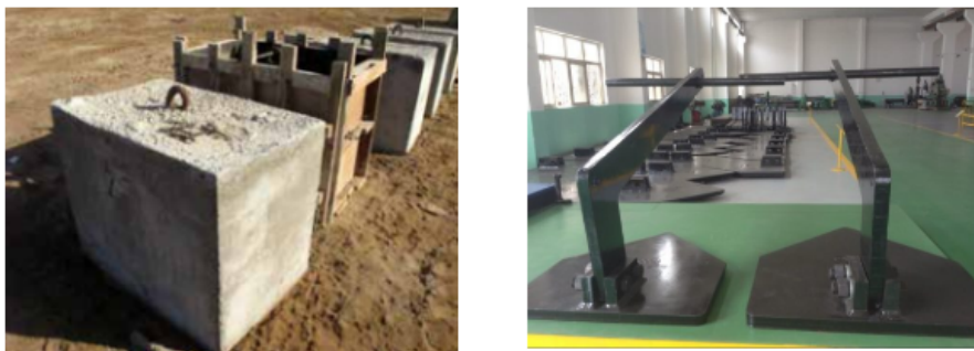
Figure 54: Dead weight concrete anchor solution to the left and plough anchor to the right [5] [28]
