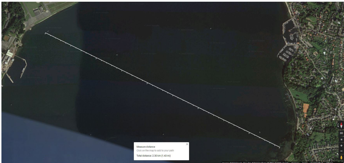
Figure 8.3: The fetch at the OS in the Bight of Kiel given east-south-easterly winds is 2.3 km (Google, 2019)
