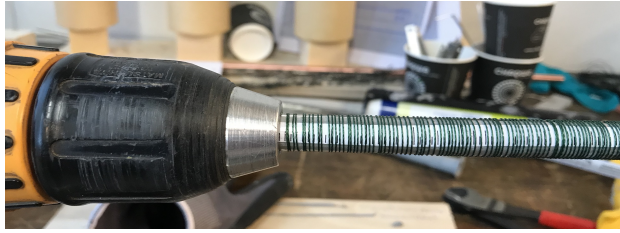
(a) Thread spun around tube and rod
