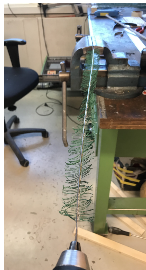
(b) Drilling of steel rods with fouling
