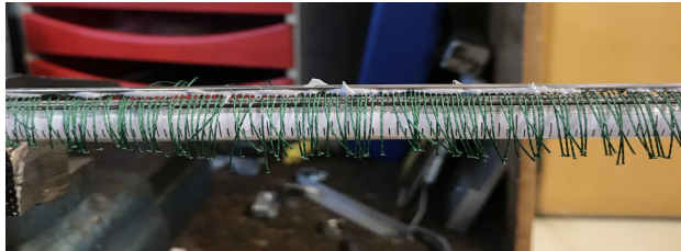
(b) Thread cut and steel rods glued
