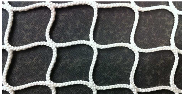
Figure 2.1: Rachel knot less knitting. (Klebert et al., 2012)
