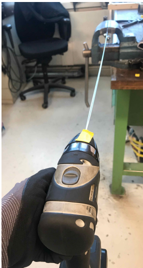
(a) Drilling of clean steel rods
