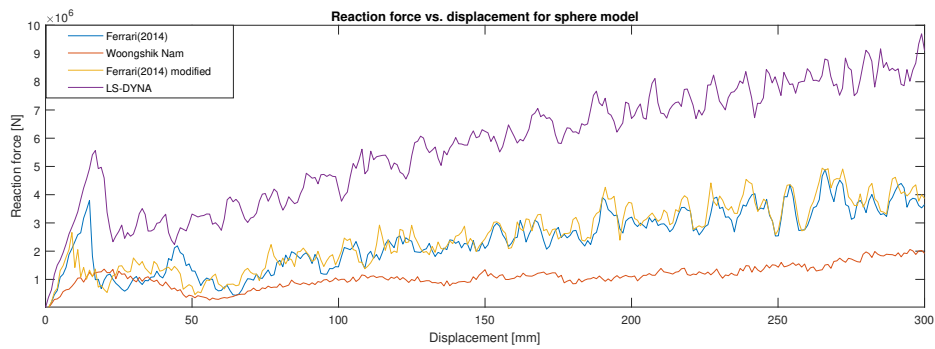
Figure B.1: Comparison of the force versus displacement of the material models in the project thesis.
