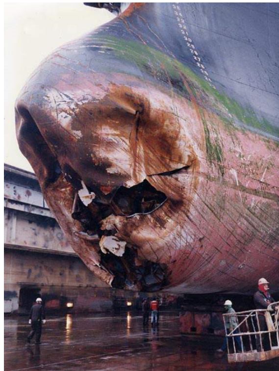
Figure 1.1: Bow damage of Overseas Ohio due front collision with iceberg (Hill, 2006).
