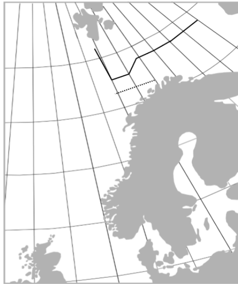
Figure 2.1: Probability of collision with iceberg at the Norwegian Continental Shelf. Solid line and dotted line indicates probability of exceeding of 10^{-4} and 10^{-2} , respectively(NORSOK, 2016).
