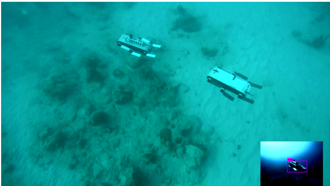
FIGURE 1.8: Hexapod Underwater Visual Target Tracking Using YOLOv2[21]
