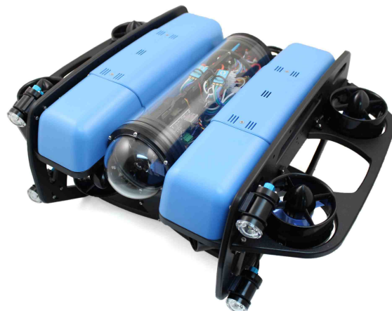
FIGURE 3.3: BlueROV2 Heavy Configuration[35]
