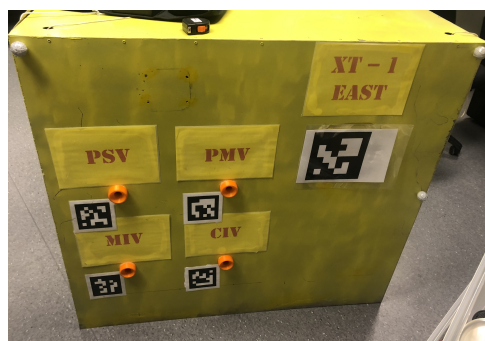
Figure 6.5: AruCo marker attached to the yellow metal box serving as a background template for underwater images
