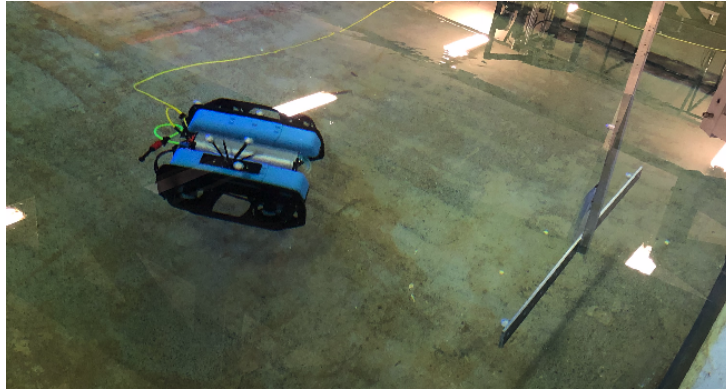
Figure 6.1: Laboratory setup illustrating the BlueROV2 together with a target object attached to the template metal stick in the MC-lab pool
