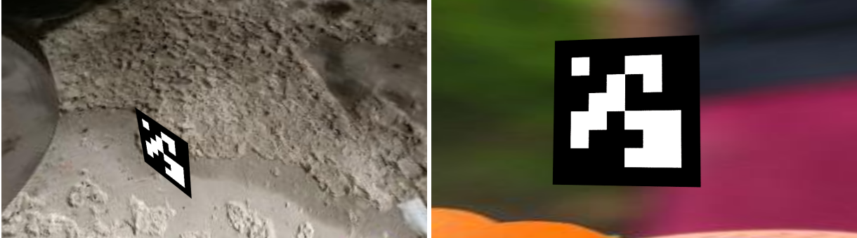
Figure 5.2: Samples from the simulated dataset containing images of the Aruco marker taken from different camera poses
