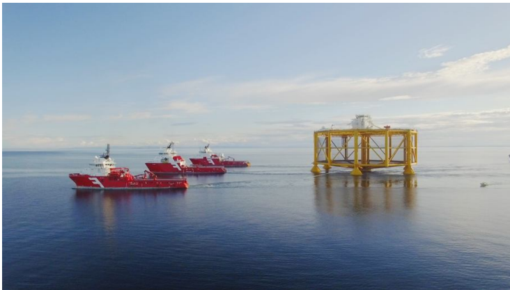
Figure 2.6: Ocean Farm 1 towing operation [20]
