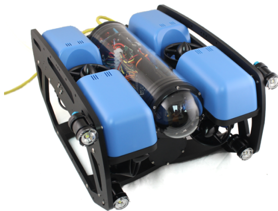
Figure 4.1: BlueROV2 by BlueRobotics [1]
