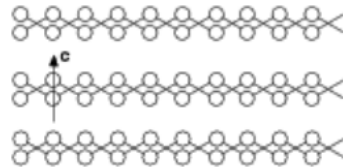
(b) Horizontally arranged basal planes with a vertical c -axis
