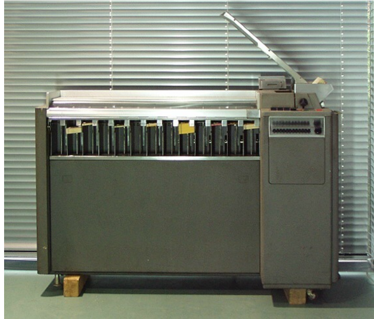
Figure 2.2: A sorting machine for punch cards [14].
