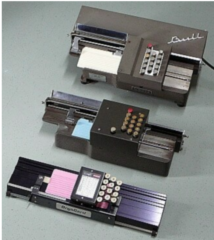
Figure 2.1: A punching device to punch holes in a punch card [14].
