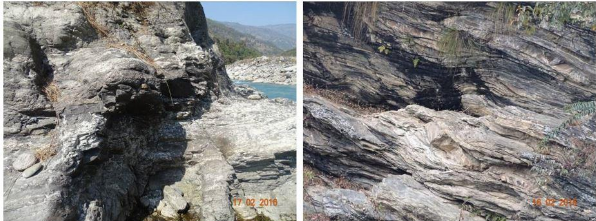
Figure 4-5 Outcrop and close view of green phyllite with quartzite intercalation at Powerhouse (Hydro-Consult 2016)
