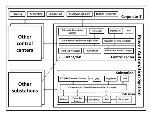
Figure 2. A typical power automation system. SCADA, supervisory control and data acquisition; EMS, energy management system; HMI, Human Machine Interface; IED, Intelligent Electronic Device.
