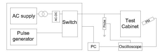
Figure 5.1: Test setup for fast rise time repetitive pulses
