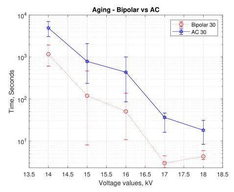
Figure 6.5: Aging - Bipolar vs AC
