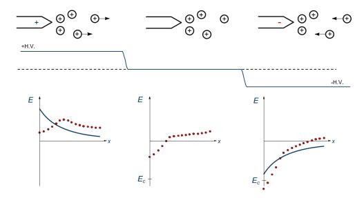
Figure 6.11: Field enhancement from space-charge, alternating polarity [26]
