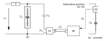
Figure 4.4: Coupling device in series with the coupling capacitor [8]
