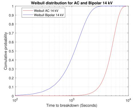
Figure 6.6: Weibull distribution for AC and bipolar 14 kV
