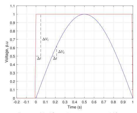
Figure 6.9: Illustration of the differences between square wave and AC
