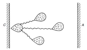
Figure 3.4: Secondary avalanche generated by photoelectrons [9]
