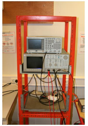
Figure B.1: Measure and signal generator setup for AC sinusoidal
