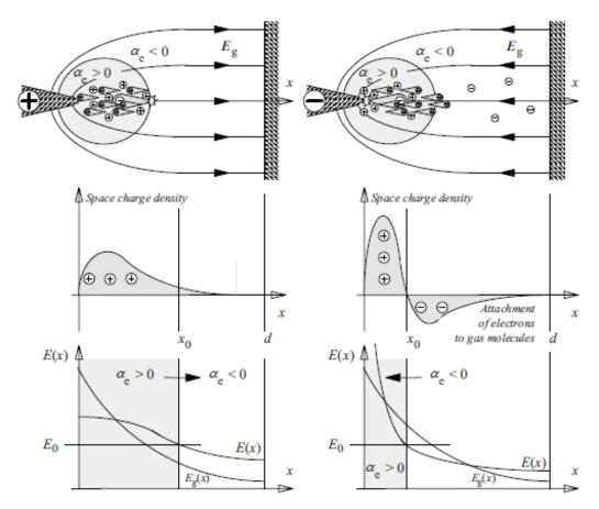
Figure 3.5: Polarity effect for positive and negative electrode [9]
