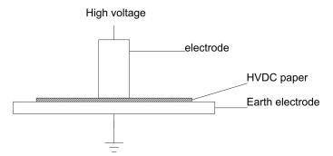
Figure 5.4: Illustration of the test object for fast rise time repetitive pulses
