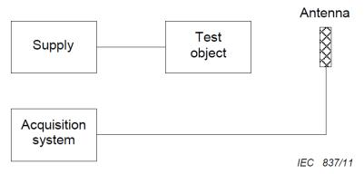
Figure 4.8: Antenna located nearby the test object [20]
