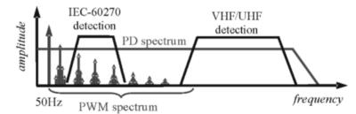
Figure 4.2: Illustration of partial discharge frequency spectrum overlapping with the PWM and detection spectrum [2]
