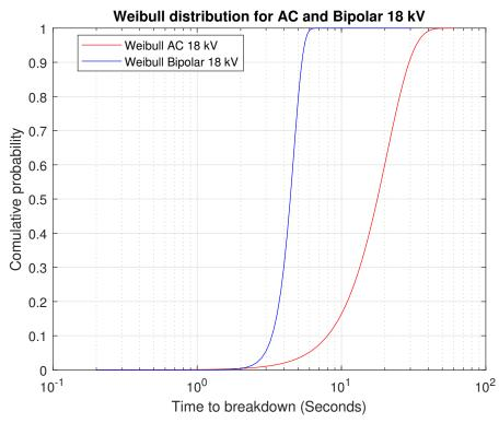
Figure 6.8: Weibull distribution for AC and bipolar 18 kV
