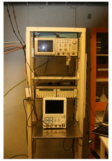
Figure A.1: Measurement and trigger setup for fast rise time repetitive pulses
