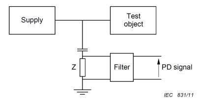
Figure 4.6: Coupling capacitor with filter [20]
