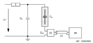
Figure 4.5: Coupling device in series with the test object [8]
