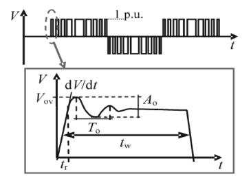
Figure 1.1: PWM sequence with the fast rise time repetitive pulses illustrated [2]
