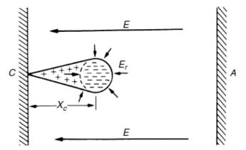
Figure 3.3: Space charge fields close to the avalanche head [9]
