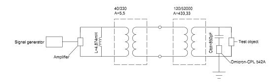
Figure 5.2: Schematics of the test setup for AC sinusoidal
