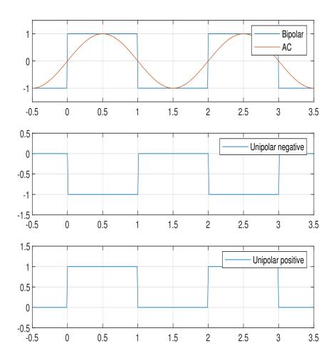
Figure 6.1: Schematic of different wave shapes
