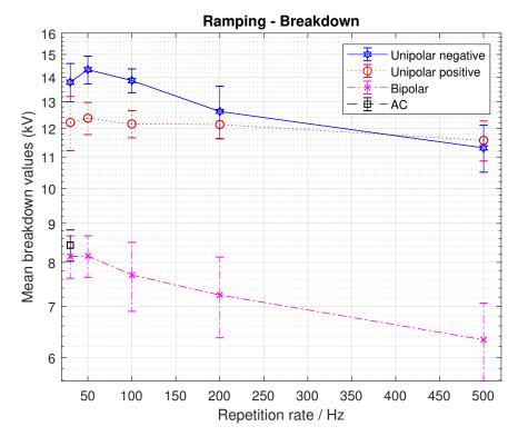
Figure 6.2: Breakdown values from ramp to breakdown, 1 kV/mm
