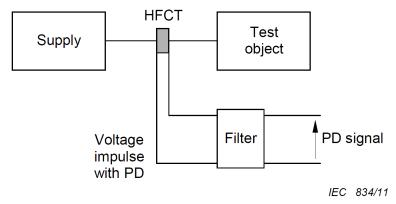
Figure 4.7: High frequency current transformer in shunt [20]
