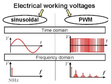
Figure 4.1: Time domain and frequency domain for PWM and sinusoidal [2]
