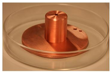
Figure 5.6: Test object for fast rise time repetitive pulses with drilled holes for banana plugs
