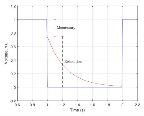
Figure 6.10: Illustration of the delay in applied voltage for fast rise time repetitive pulses
