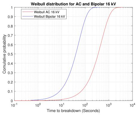
Figure 6.7: Weibull distribution for AC and bipolar 16  $\rm kV$
