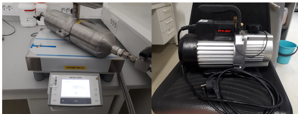
Figure 3.7: Ammonia tank, weighing scale, and vacuum pump.
