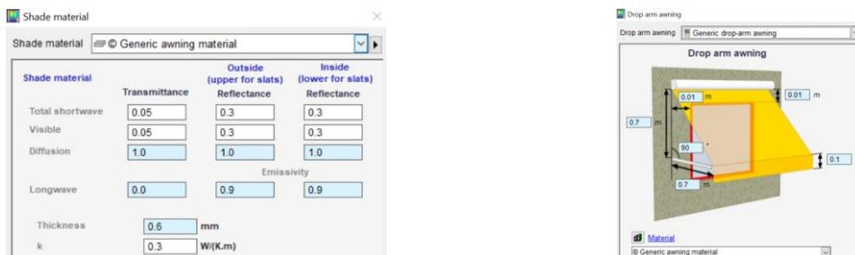
Figure 3-30 Properties and dimensions of external window shading - drop arm awning
