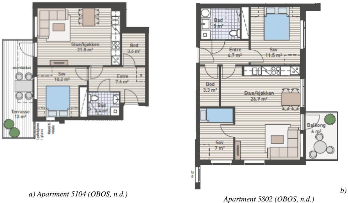
Figure 3-21 Apartment layout for the two selected zones
