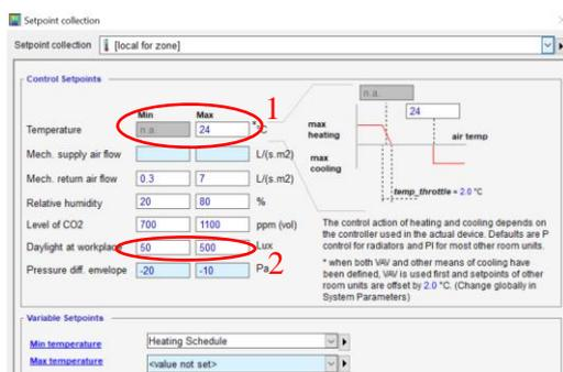
a) Control setpoints. (1) Temp. setpoints, connected to heating schedule
