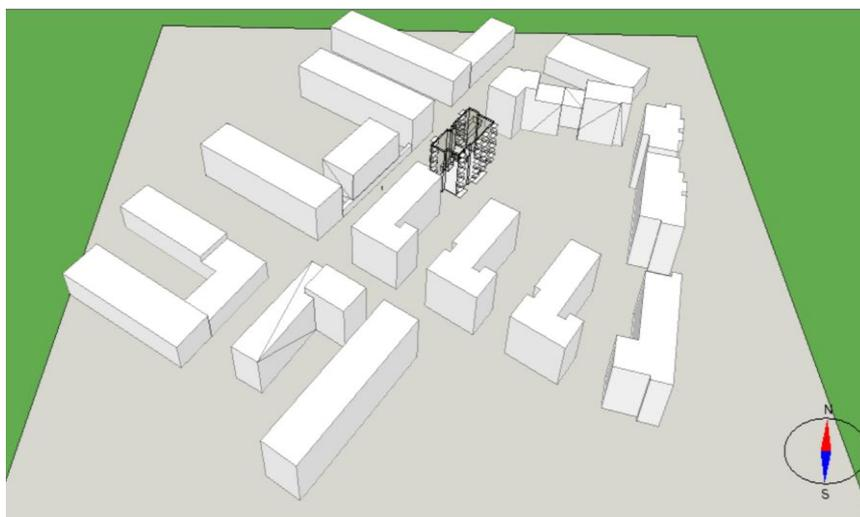
Figure 3-4 Model of project site with building case (wireframe) and neighboring buildings (white) - 3D view in IDA ICE
