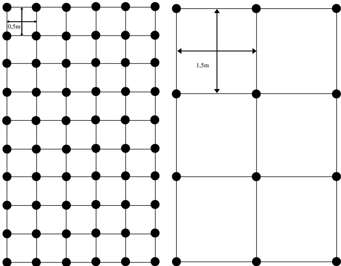
a) Min. resolution acc. to NS-EN 12464-1:2011 & default resolution in IDA ICE: 0,5m – 60 grid points
