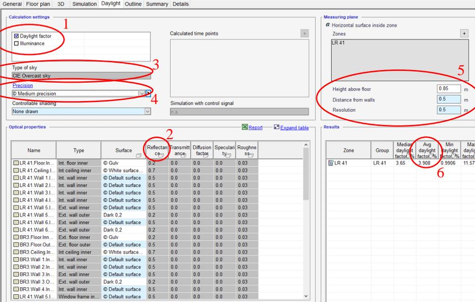
Figure 3-8 Daylight simulations tab with relevant settings and inputs circled in red
