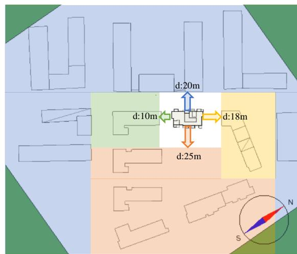
Figure 3-23 Chosen areas for calculated building heights and the distances used to calculate them acc. 45°
