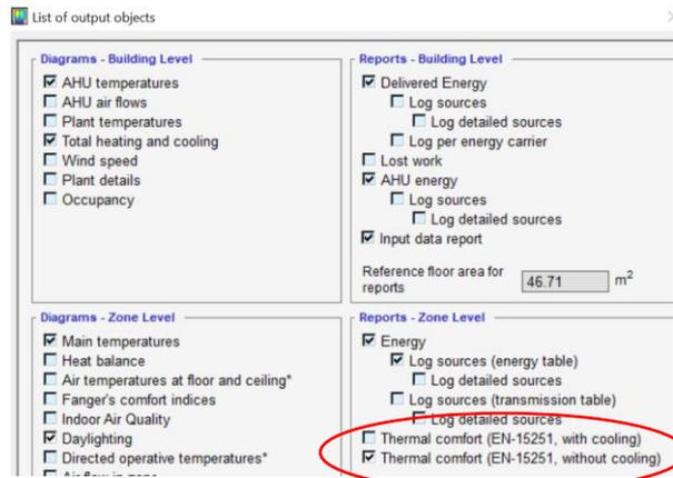
Figure 3-16 Requested output setting for thermal comfort results
