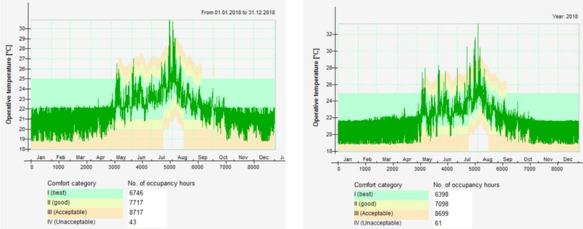
a) Top floor, glazing alt. C with no window shading or shading obstructions, Oslo
