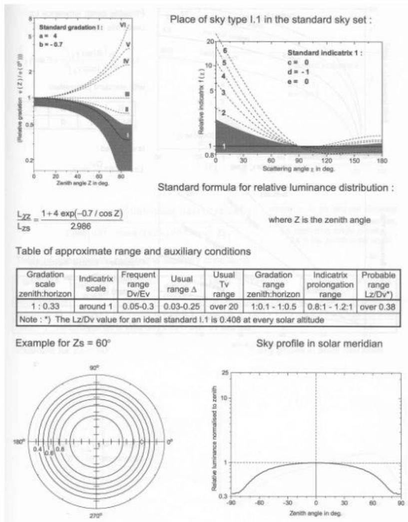
Figure B - 2 CIE sky type I.1 Overcast with steep gradation and with azimuthal uniformity (Matusiak, 2017b)
