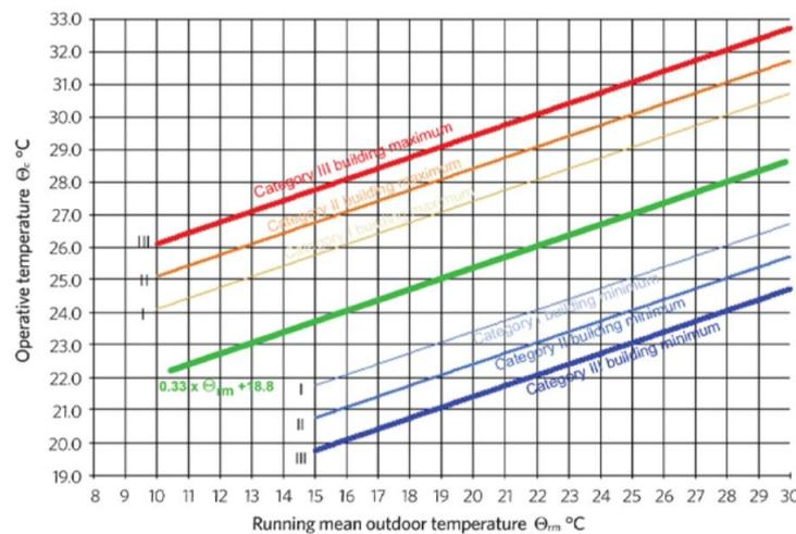
Figure 3-6 Acceptable operative temperatures ranges for free-running, naturally conditioned spaces (Dwyer, 2017)
