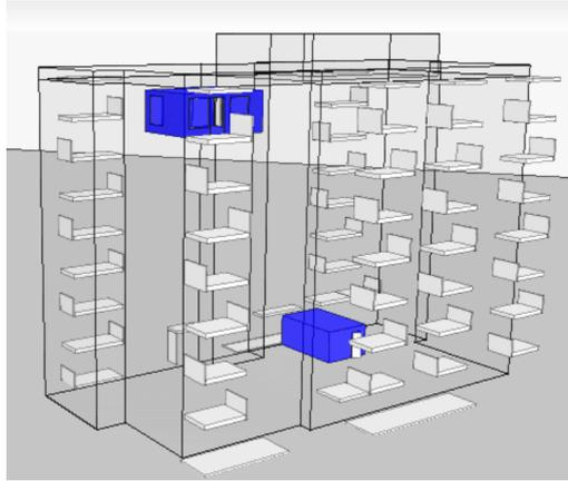
Figure 3-19 IDA ICE model made for the case study, with critical zones marked in blue and balconies as white 3D-objects
