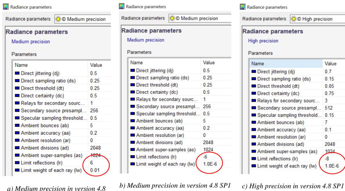
Figure 3-9 Radiance parameters for daylight simulations for two versions and precision levels in IDA ICE
