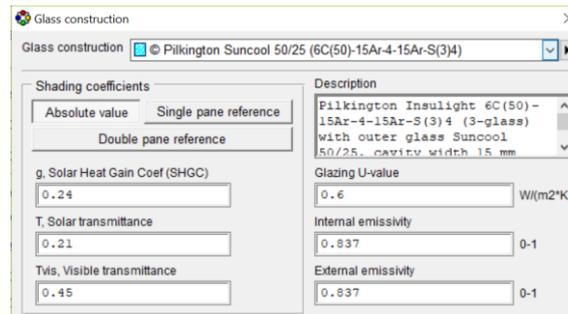
Figure 3-31 Window properties for window with additional coating - Pilkington Suncool 50/25
