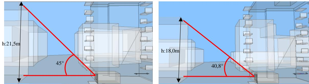
a) Maximal shading angle acc. to preaccepted performances TEK17 - 45°
