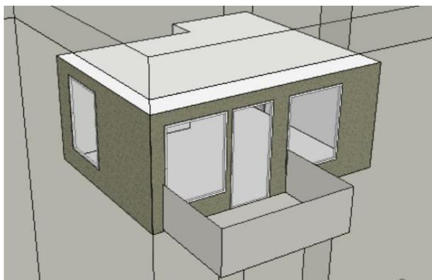
Figure 3-27 Shading object: Balcony in IDA ICE
