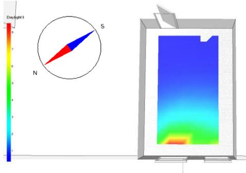
Figure 3-10 Illustration of how the results for daylight factor is animated in IDA ICE
